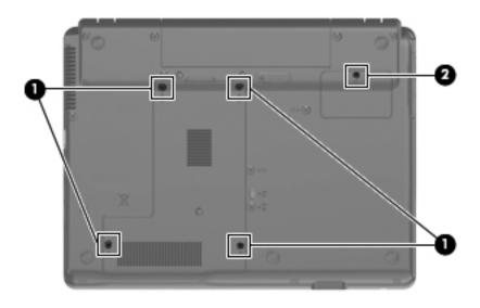
Where used: 4 captive screws 1 that secure the hard drive cover to the computer and 1 captive screw 2 that secures the wireless module compartment cover to the computer
